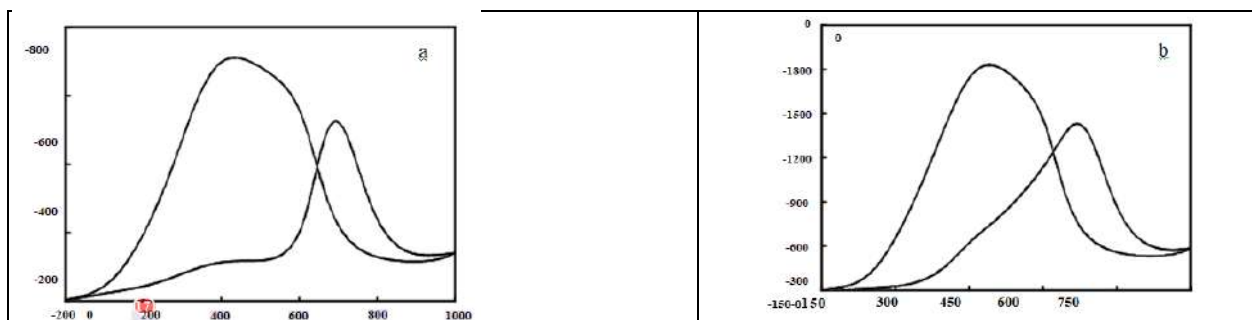
Fig. 5 Cyclic Voltammetry of (a) PoPD-Pt and (b) PoPD-Pt-Ru (1:0.25) Electrodes in 0.2 M \text{Na}_2\text{SO}_4 with 0.5 M Formic Acid at pH 1 using a Scan Rate of 5 \text{ mV s}^{-1}
